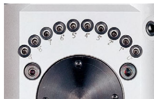
Indexing mechanism in 1° increments
