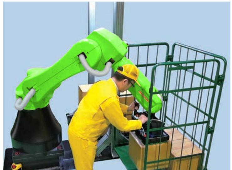
Workpiece transfer with Hand Guidance
