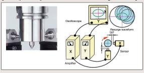
This example uses a static capacitance non-contact displacement meter. X and Y axis displacement can be measured simultaneously, with the resurge waveform displayed on an oscilloscope
