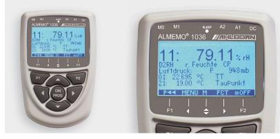
Reference measuring instruments for humidity and temperature High-precision measurement with the Pt100 psychrometer and Pt100 sensors **Resolution Temperature 0.001 K** Relative humidity 0.01 % Dew point 0.01 K
