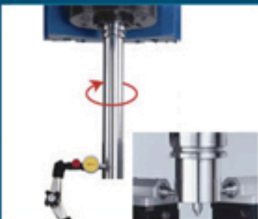
Fig. 2—Slowly rotating a precision-machined bar can measure a spindle's static runout. The non-contact measurement device below can evaluate runout at the spindle's operational speed.
