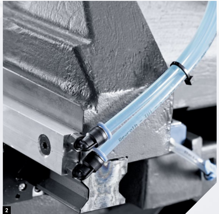
1+2: Cooled ball screw nuts and guideways 3: Optimal overview of and accessibility to the hydraulics
