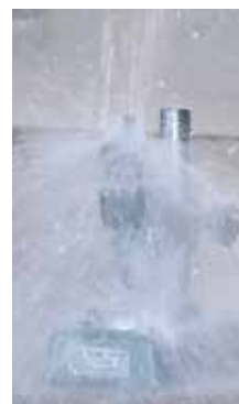
Rated to IP66 water- and dust-proofing standard and oil resistance improved.
