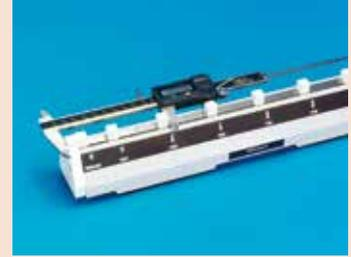
Checking accuracy of caliper (outside measurement)
