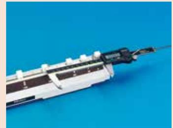
Checking accuracy of caliper (inside measurement)
