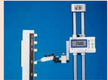
Checking accuracy of height gage
