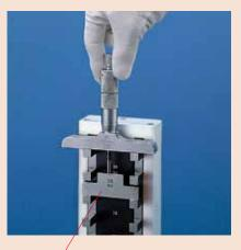
A 25 mm anvil block provides the reference surface for the depth micrometer rod
