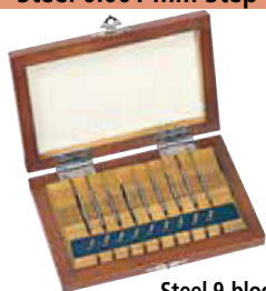
Steel 9-block set (1.001 - 1.009 mm)
