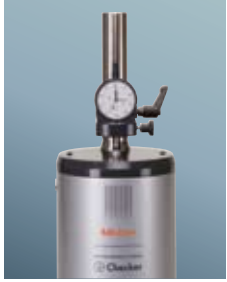
Inspection using analog type indicator
