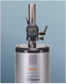
Inspection using digital type indicator
