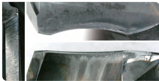
After 2,500 pieces of machining (5 holes / piece)
