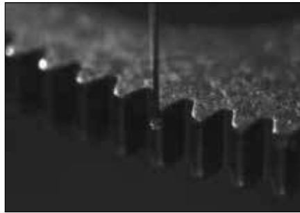
Measurement using the MPP-NANO 0.125-mm-diameter stylus
