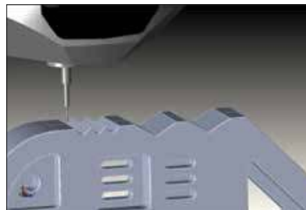
Creating nominal sections from CAD data (CAT1000S)
