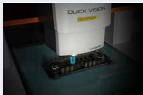
Example of measuring an engine control unit
