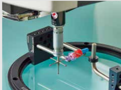
Example of measuring a valve used in medical equipment
