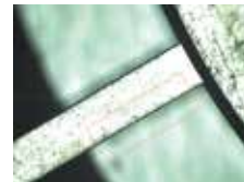
Positive edge detection with co-axial light
