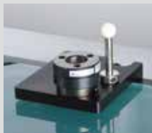
Master ball (optional) Used for diameter compensation of the stylus.
