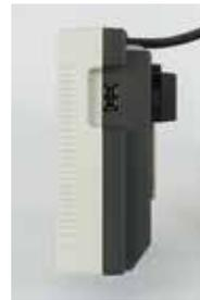
The display unit features USB2.0 Type A socket. Test results, statistical calculation results and test conditions can be saved as text data, and graphs can be saved as image data to a USB memory device.
