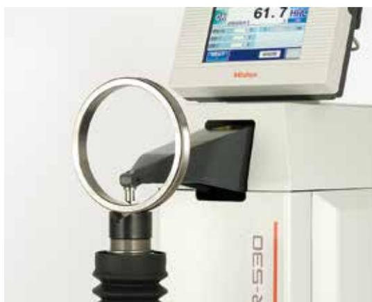
Hardness testing of internal surfaces, which previously was impossible without sectioning, is now possible. (All models.)
