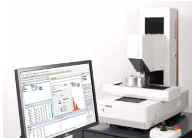
**AVPAK**, using part programs, enables automated multi-point testing.
