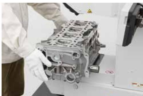
Large workpieces such as cylinder blocks can be mounted on the table as is. Testing of heavy workpieces weighing up to 100 kg is supported.
