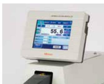
The touch-screen display unit can be mounted on top of the tester, providing significant convenience if the machine installation space is restricted. (All models.)
