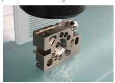
The LED used as the light source of the displacement sensor has an auto-brightness control function that enables seamless measurement of materials with different reflectivity.
