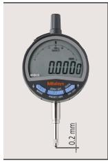
Repeatability in the range of 0.2 mm from the lowest rest point is not guaranteed for Digimatic indicators. When setting the origin or presetting a specific value, be sure to lift the spindle at least 0.2 mm from the lowest rest point.
