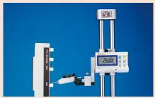
Checking accuracy of height gage
