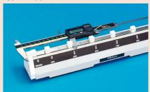
Checking accuracy of caliper (outside measurement)
