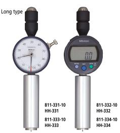
• Hardness measurement by durometer is simply performed by holding the instrument against the surface of a specimen and reading the indicated value. This type of hardness tester is most widely used for hardness testing of sponge, rubber, plastics and other soft materials.
