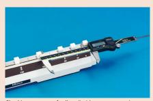
Checking accuracy of caliper (inside measurement)
