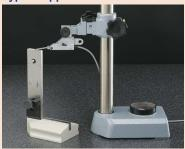
Setting a dial test indicator to a long-gaugeblock stack attached to the base with a D-type connector
