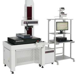
**SV-C4500CNC** (Contour detector shown mounted together with the inclinable drive unit and Y-axis table)
