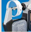
Parallelism can be estimated using an optical parallel held between the faces. First, wring the parallel to the anvil measuring face. Then close the spindle on the parallel using normal measuring force and count the number of red interference fringes seen on the measuring face of the spindle in white light. Each fringe represents a half wavelength difference in height (0.32  $\mu$ m for red fringes).
