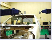
Measurement example for dual-ram type (Simultaneous use of touch-trigger probe and line laser probe)
