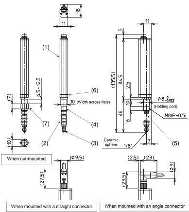
When connecting the connector, engage it firmly and tighten the threaded part securely. (Recommended tightening torque:  $0.2\ to\ 0.3\ N\cdot m)$
