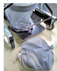
Pull down polybag for a next dust accumulation space
