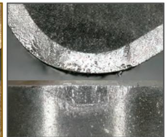
Conventional Tool (Uncoated) (After Cutting 2.5km)
