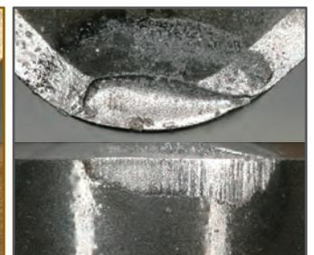
Conventional Tool (Uncoated) (After Cutting 0.5km)
