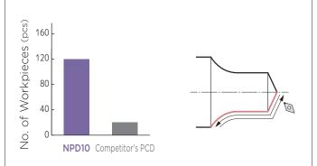
Tool: DCMW11T302 (NPD10) External Turning Cutting Conditions: vc = 30m/min f = 0.01mm/rev ap = 0.1mm Dry
