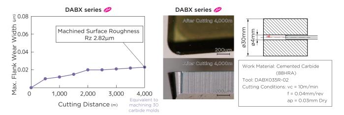
Minimal wear even after cutting distance of 4,000m
