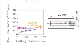
Tool: DABX035R-02 (NPD10) Internal Boring Cutting Conditions: vc = 10m/min f = 0.05mm/rev ap = 0.025mm Dry
