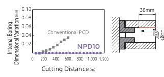
Work Material: Cemented Carbide VM30 (91HRA) Tool: DCMW11T304RH Cutting Conditions: vc = 20m/min f = 0.05mm/rev ap = 0.05mm Dry
