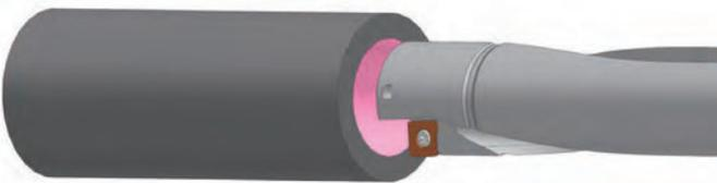
Deep hole drilling of H75mm from both ends
